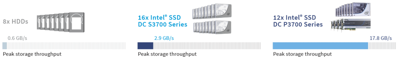
Figure 2: The peak disk throughput in GB per second for each solution. Larger numbers are better.
